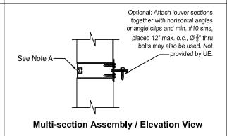
Note A: After the louver is secured to the substrate, install backer rod and caulking (not provided by UE) around the perimeter of the louver to the substrate and at section joints where possible. If mullion strips are provided, place caulk behind mullion strip (if possible) before attaching. If mullion strip is already installed, apply a small bead where it touches the louver.
